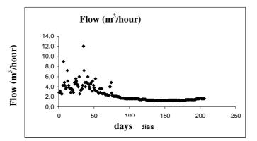
Fig. 3 – Leachate's flow rate from January to August of 2002. Source: Autor
